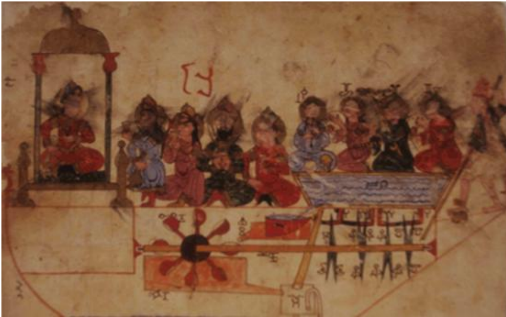
Figure 5: An illustration by al-Jazari of the internal mechanics of an automated boat: al-Jazari 1974, category II, chapter 4, p. 107. Held at the Topkapi Palace Museum Library in Istanbul, al-Jazari, Al-Jami' bayn al-ilm wa'l-amal al-nafi fi sina'at al-hiyal , MS Ahmet III 3472.
