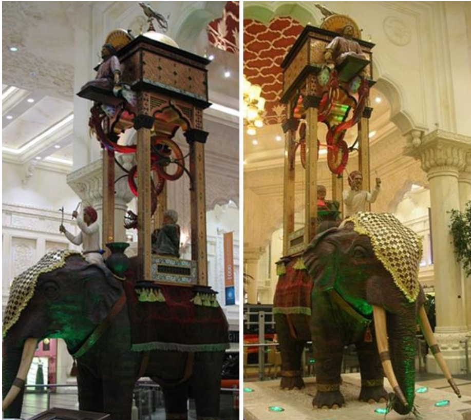
Figure 2: Two photos of the fascinating reproduction of the 8.5 meters high elephant clock of al-Jazari in the Ibn Battuta Mall, Dubai. This was the first clock in which an automaton reacted after certain intervals of time. In the mechanism, a humanoid automata strikes the cymbal and a mechanical bird chirps after every hour. See: http://muslimheritage.com/topics/default.cfm?ArticleID=466 and http://muslimheritage.com/topics/default.cfm?ArticleID=188 .
