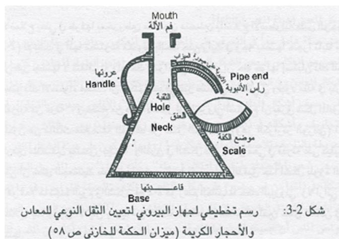
Fig. 3 A sketch of Al-Biruni apparatus which he used to determine the specific gravity of gems and minerals.
